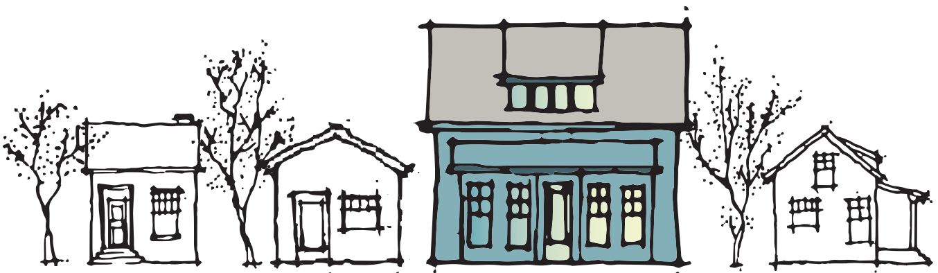
Figure 1: Small lot subdivision development should follow the established size, shape, and form of the surrounding neighborhood through the use of similar proportions and details. In this example, the house in color is disproportionate in scale compared to the surrounding houses.
