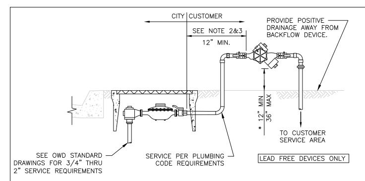
\*IF THE BACKFLOW PREVENTION DEVICE TO BE INSTALLED IS OF THE TYPE KNOWN AS A "VACUUM DEVICE", IT SHALL BE INSTALLED A MINIMUM OF 12" ABOVE THE HIGHEST POINT OF USAGE DOWN— STREAM FROM THE DEVICE.
