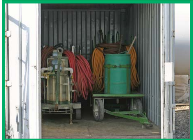
Example of a container used to store pesticide application equipment reducing the chance of pesticide residues from being washed off during storm events.
