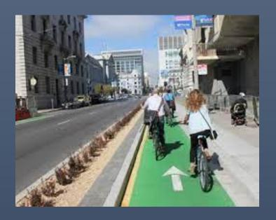
Class IV - Cycle Tracks (Class IV) provide a right-of-way designated exclusively for bicycle travel within a roadway and which are protected from other vehicle traffic with devices, including, but not limited to, grade separation, flexible posts, inflexible physical barriers, or parked cars.
